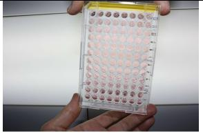
When backlit, there are no fractures or cracks visible below
