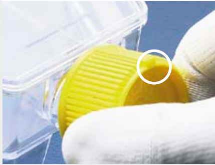
VENT position at 12 o'clock = gas exchange
